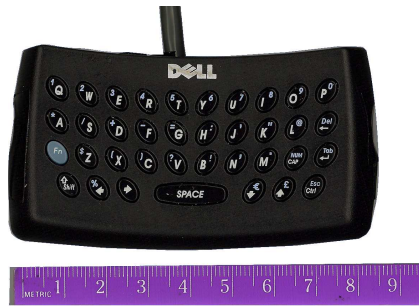
Figure 2: The Dell mini-QWERTY keyboard used in both studies.
